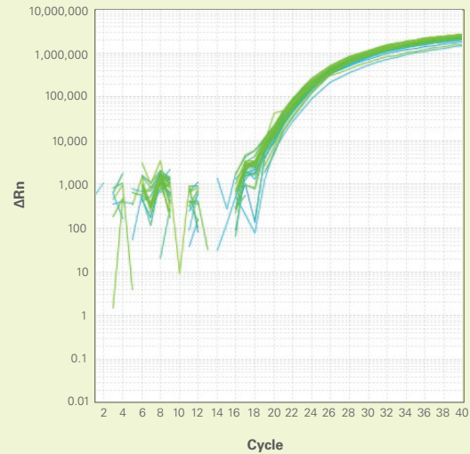
Figure 11. Ideal Amplification Properties for Successful HRM Analysis.
