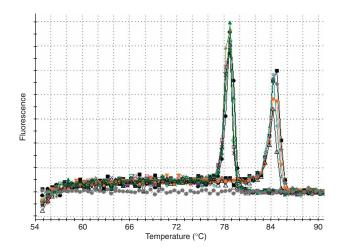
**Figure 10** | SYBR Green melt curve demonstrating the co-amplification of an mRNA target (lower  $T_m$ ) and genomic DNA with a short intron. The identity of the peaks can be determined from the  $T_m$  without the need for sequencing.
