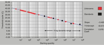
**Figure 5** Acceptable and unacceptable standard curves. All the unknowns (red dots) in the upper picture are contained within the dynamic range of the standard curve, which is demarcated by the two outermost points of the standard represented by black dots. This allows accurate quantification of the corresponding mRNAs. In the lower picture, a majority of the unknowns is below the highest dilution of the standards  $(4 \times 10^3 \text{ copies})$ .
