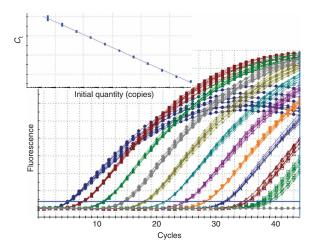
**Figure 7** | The relationship between amplification plot and standard curve. The amplification plots were generated by serial ten-fold dilutions of an RNA sample containing  $3 \times 10^{11}$  targets. Eight replicates were run for each dilution point. The horizontal blue line marks the threshold, at which the  $C_{\rm t}$  values are obtained. The standard curve (insert) generated from these amplification plots is linear over 11 logs, with a slope of -3.323 and an  $R^2$  of 0.999.
